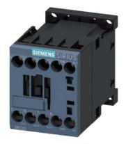
power contactor, AC-3e/AC-3, 16 A, 7.5 kW / 400 V, 3-pole, 230 V AC, 50/60 Hz, auxiliary contacts: 1 NC, screw terminal, size: S00  $\,$
